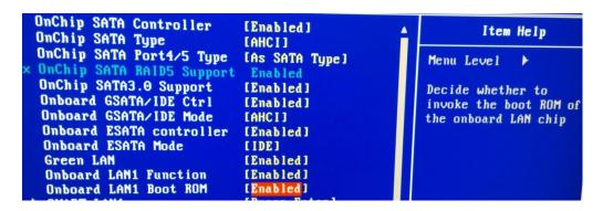
On booting the client system select the PXE boot option, e.g. Realtek PXE B05 in our test case:
