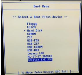
The Network Interface card on the PC will then broadcast to find a PXE server on the network, once found press F12 to boot from the PXE server:
